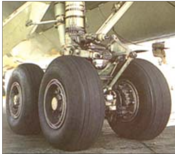
Main wheels on the undercarriage of an airliner. Air plane landing gears and wheels need to bear high stresses and shocks.
