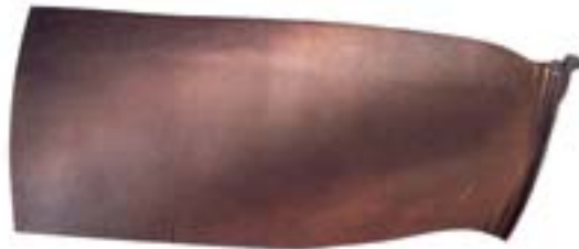
This is a fan blade from a jumbo jet engine. On take-off, the stress on the metal is immense, so to prevent the fan from flying apart, the blades must be both light and very strong. Titanium, though expensive, is the only suitable metal.
