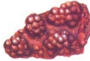
Haematite is an ore of iron. It often forms kidney-shaped lumps, These give the ore its nickname of kidney ore.
